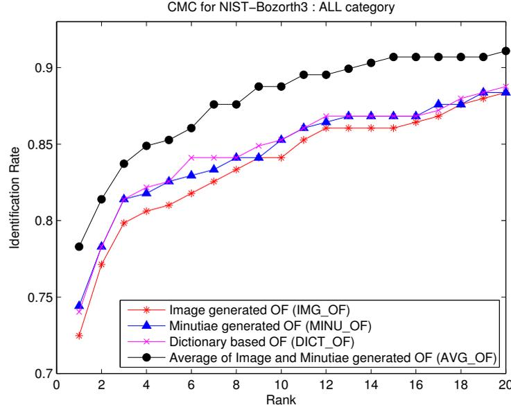
**Figure 3.6:** CMC curve showing the rank identification rate of NIST-Bozorth3 for NIST-SD27 when different types of OF estimation techniques were used for the tenprints, and *MANUAL\_OF* for latents, when applying the proposed OF-based pre-alignment.
