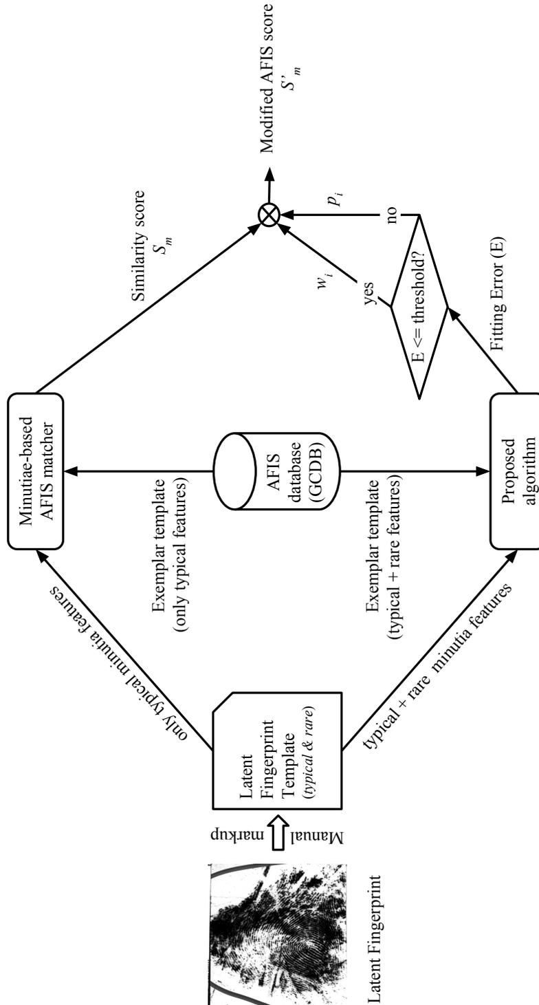
Figure 5.3: Sequence of steps in estimating the modified similarity score of a reference minutiae-based matcher.
