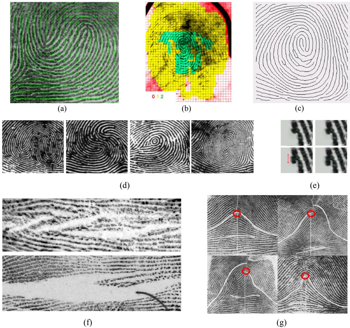
**Figure 4.2:** Some example Extended Feature sets [Hicklin, 2007]: (a) ridge flow maps, (b) local ridge quality, (c) ridge path, (d) pattern classifications, (e) protrusions, (f) flexion creases, (g) center point of reference.
