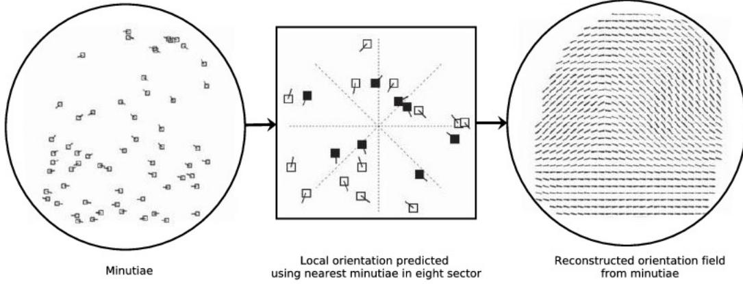
**Figure 3.4:** Minutiae based orientation field reconstruction [Feng and Jain, 2011]. The solid black boxes are the nearest minutiae in each sector.
