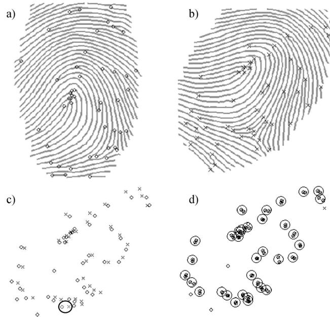
**Figure 2.2:** A generalized Hough transform based alignment. a) and b) shows the minutiae extracted from input and reference fingerprint; c) input and reference minutiae superimposed; d) circles denotes minutiae pairs mated using generalized Hough transform technique [Maltoni et al., 2009].
